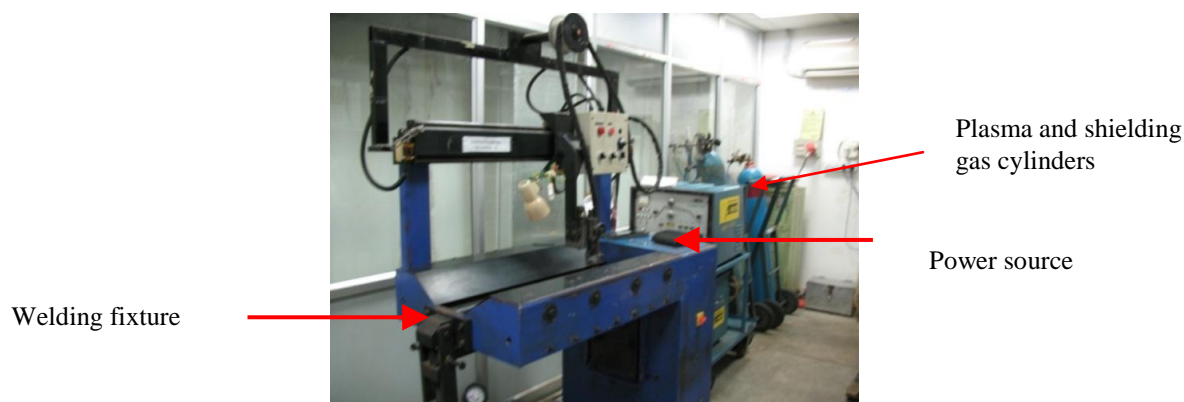
Figure 1. Micro Plasma Arc Welding Setup.
