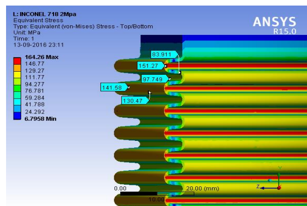
Fig. 19 Stress distribution at Pressure 20 Bar
