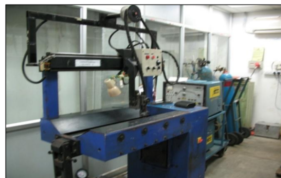
Fig. 1. Micro-plasma arc welding setup.
