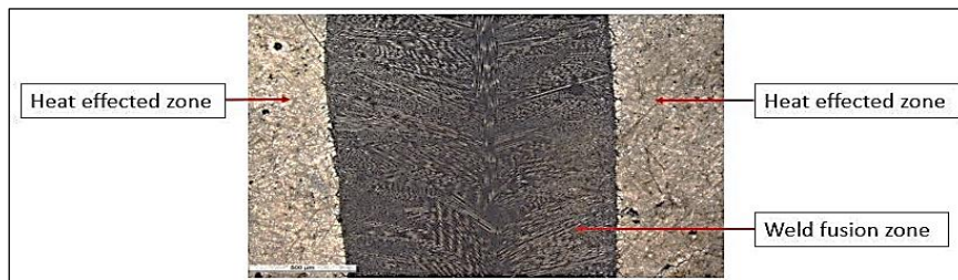
Fig. 4. Microstructure of weld fusion zone and HAZ.
