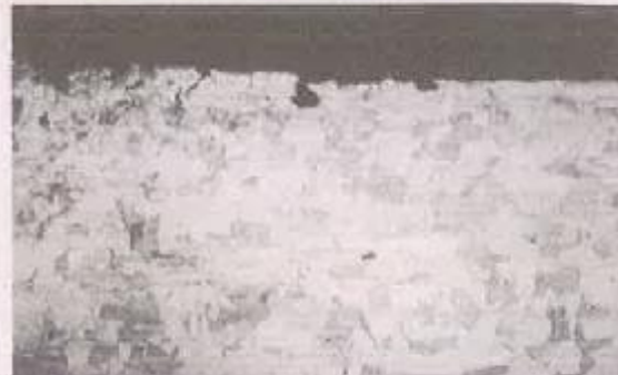
Pitting corrosion observed on cut cross section of a cupro-nickel tube from a turbine lub-oil cooler
