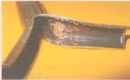
Pitting corrosion observed on cut cross section of a cupro-nickel tube from a turbine lub-oil cooler
